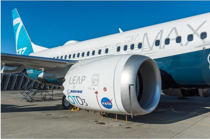
737 LEAP-1B Inlet Liner Flight Test (Summer 2018)
