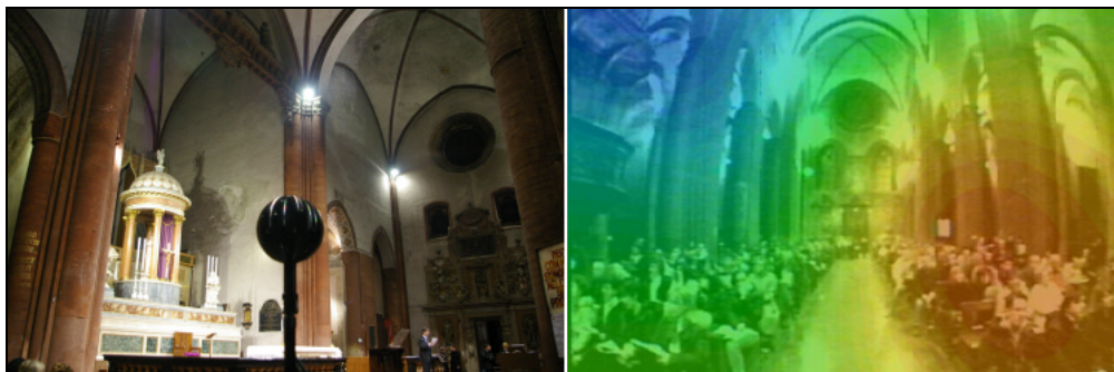
Fig. 8: Measurement inside an old church. Sensor (left) and noise maps (right)
