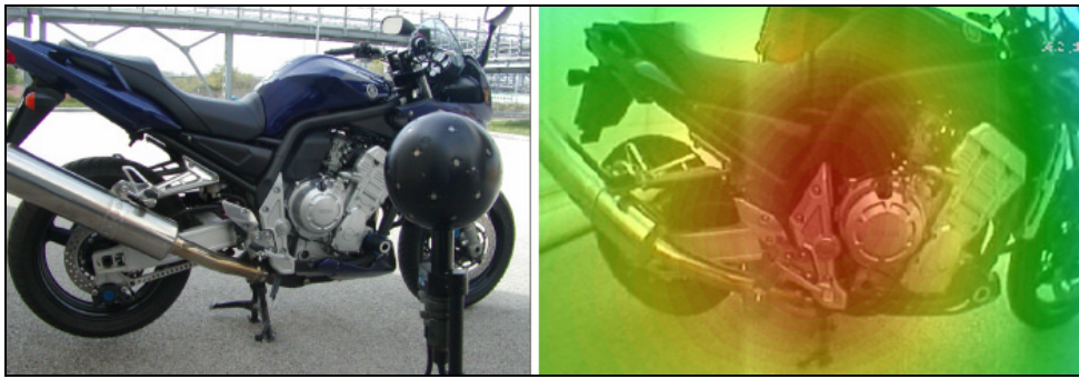
Fig. 11: Measurement on motorbike at given rpm. Sensor (left) and noise maps (right)
