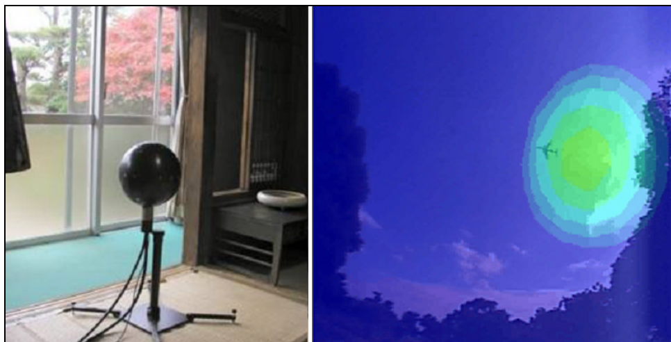
Fig. 7: Noise map in front of a window. Sensor (left) and noise maps (right)
