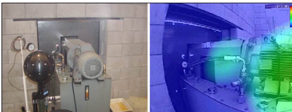
Fig. 10: Measurement inside an old church. Sensor (left) and noise maps (right)
