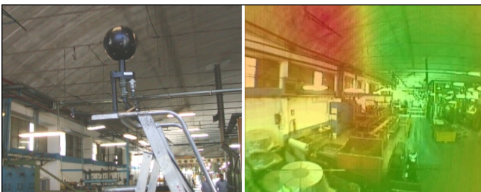
Fig. 4: Noise map inside industrial building. Sensor (left) and noise map (right)
